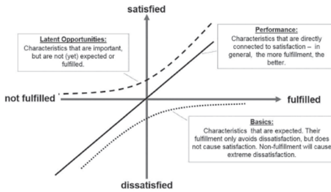
Figure C.1 — Relationship between various characteristics and customer satisfaction
